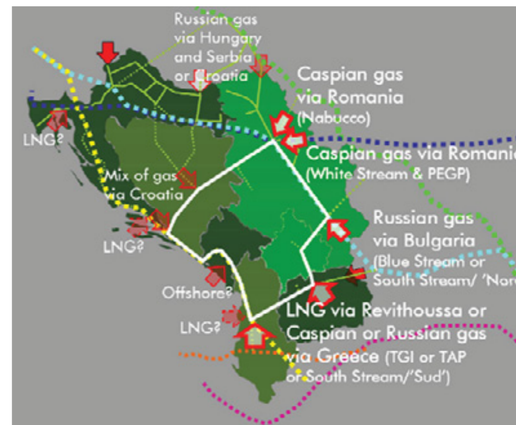
Fig 6.1 The Energy Community Gas Ring concept" (Source: The study of gasification of the region of South East Europe)
