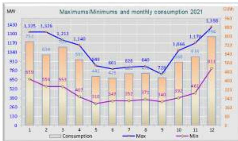
Fig. 2.12 Monthly average of maximum and minimum load for 2021
