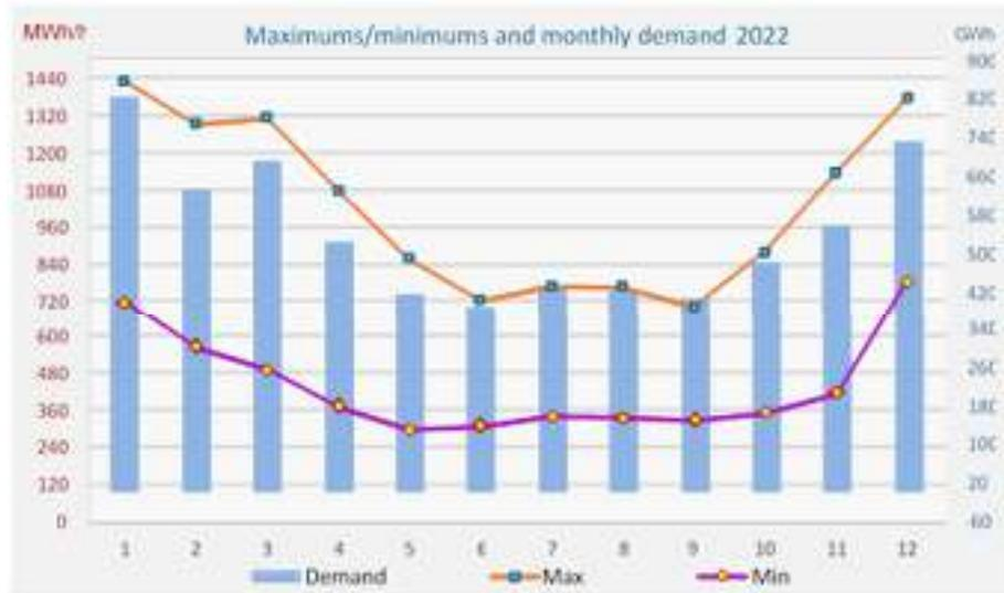
Fig. 2.13 Monthly average of maximum and minimum load for 2022
